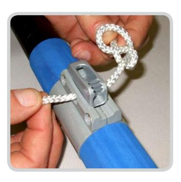
Peed the 5mm rope through the small pulleys, then return to through the cleat and tie a figure of eight knot to prevent the rope from coming back through the cleat.
