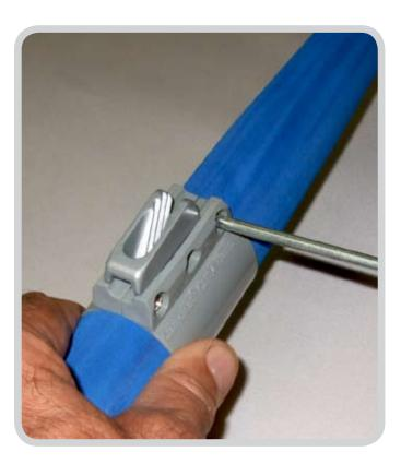
03 When the plastic clam cleat band is on, feed the 5mm rope through the hole in the middle of the cleat and secure the ends with a figure of eight knot. Secure the knot on the outside of the boom.
