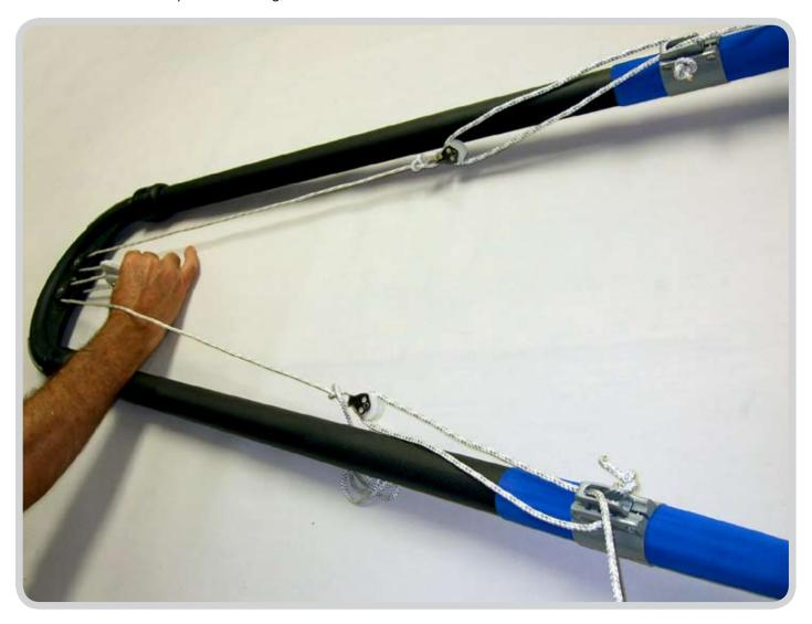
Then make a loop around the clew ears on the sail, back to the outside of the lower center pulley, around and back to the clew ears. Next go around the other top pulley and finish by tying the 4mm rope to the small pulley on the other side of the boom.
